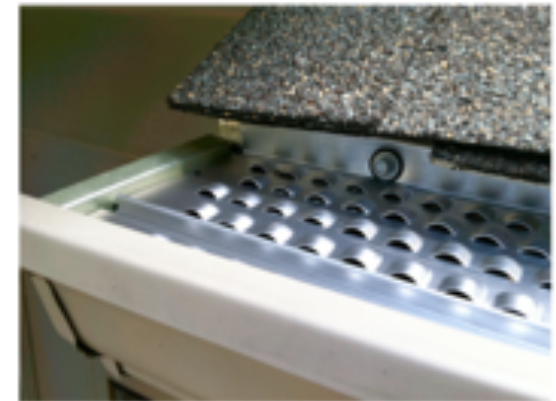
The neoprene washer used on the factory supplied ceramic coated anchor screws pulls the back wall securely against the fascia board.
